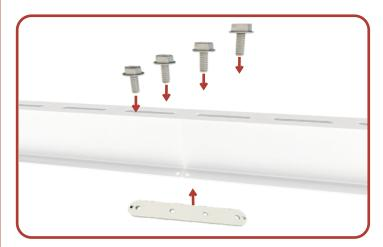
Mount the Channel Rails by rotating the Slide Nuts 90 degrees inside the Support Rails.
